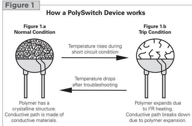
The increase in volume during melting of the crystalline phase separates the conductive particles resulting in a large non-linear increase in the resistance of the device.
